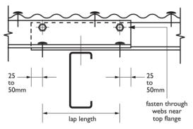
Top hat overlaps (or non-structural laps) are recommended to be a minimum of 100mm in length. In these cases structural continuity must not be assumed. When connecting overlapping top hats, place foot onto upper section to nest sections prior to and during fixing. Laps must be fastened through both webs as shown.
